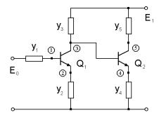
Fig. 4 Two-stage transistor amplifier
