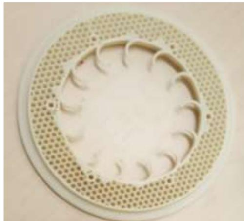
Figure 14. Airless wheel assembly installed on the Xiaomi Mijia M365 electric light scooter
