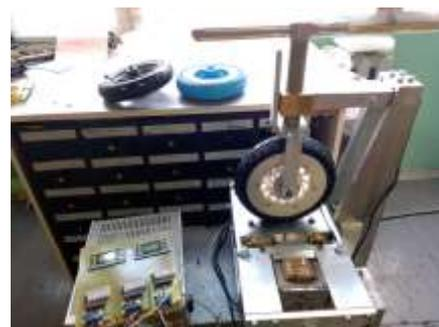
The coefficient  $C_z$  of tire's normal stiffness is the first derivative of the normal wheel load  $P_z$  with respect to the normal tire deflection  $h_z$ :
