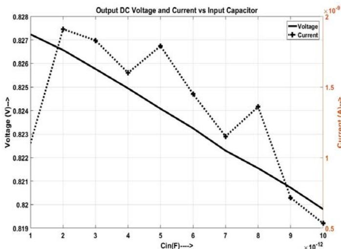
**Figure 4: Output DC voltage and current vs  $C_{in}$**
