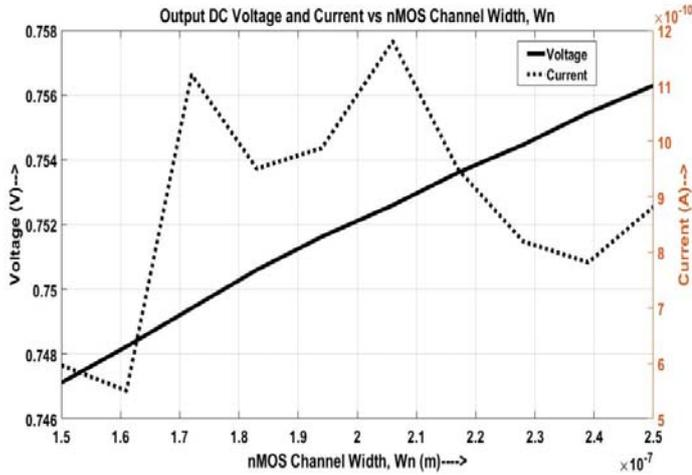
Figure 7: Output DC voltage and current vs  $W_n$
