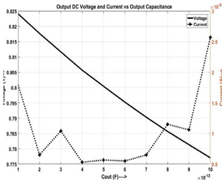
**Figure 5: Output DC voltage and current vs  $C_{out}$**
