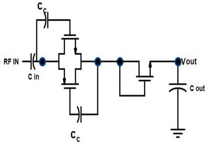
**Figure 2: Proposed 3-transistor rectifier with threshold voltage compensation**
