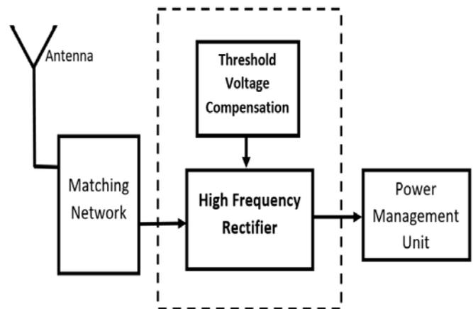
**Figure 1: The Block diagram of Proposed RF EH system**
