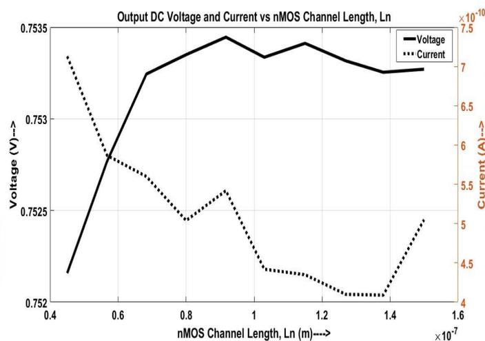
**Figure 6: Output DC voltage and current vs  $L_n$**
