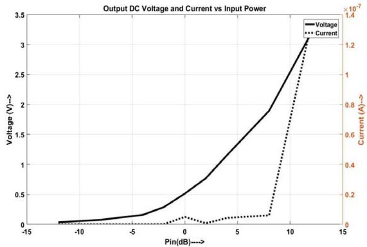
**Figure 14: Output DC voltage and current vs  $P_{in}$**
