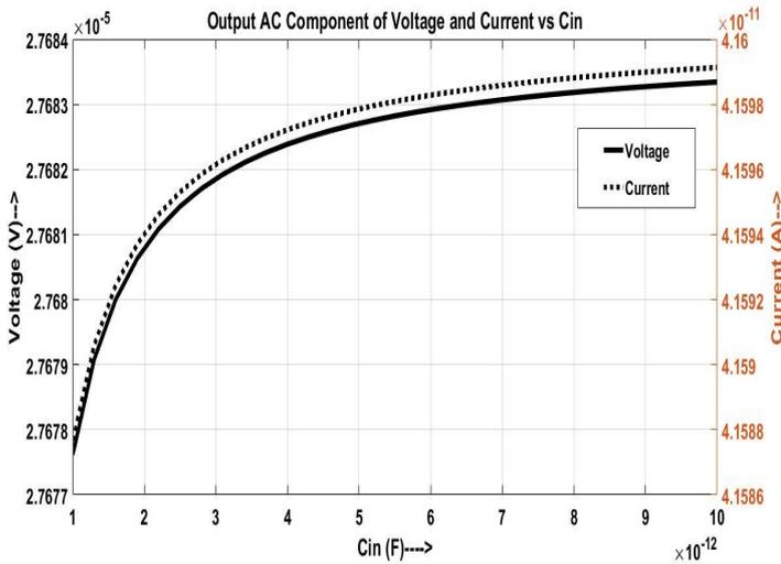
**Figure 12: Output AC components of voltage and current vs  $C_{in}$**
