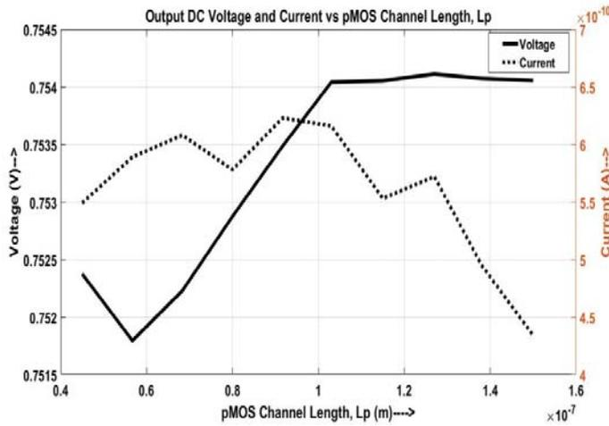
Figure 8: Output DC voltage and current vs  $L_p$
