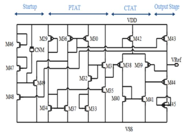
Fig 4. Schematic of the proposed band gap reference circuit [7]
