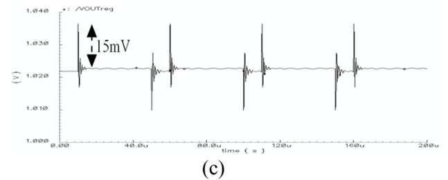
Fig 10. Load transient response of the proposed LDO regulator in different corners, (a) Typical-Typical, (b) Slow-Slow and (c) Fast-Fast
