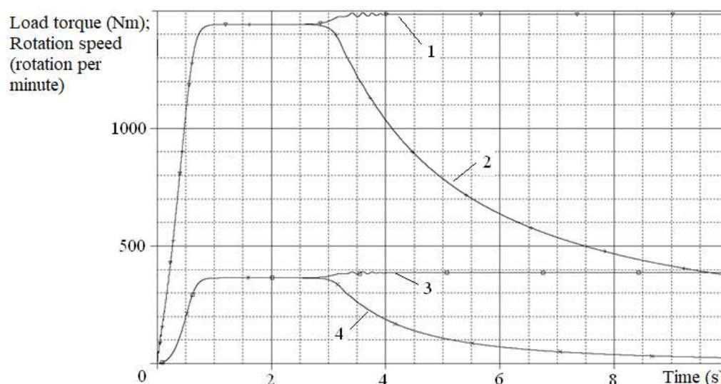
Fig. 2: Instability of joint operation of a pair of series connected IMs with completely identical parameters. Results of simulation of rotation speeds (graphs 1 and 2) and load torques (graphs 3 and 4) of two NVA-55 IMs. Graphs 1 and 3 refer to one IM, 2 and 4 to another IM
