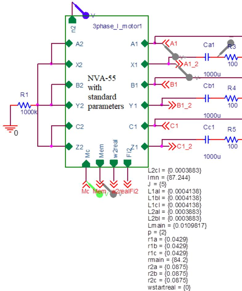
Fig. 3: OrCAD hierarchical block symbolizing the computer model of the IM of type NVA-55. In capacitive dividers, 100 Ohm resistances are connected in series with 1000  $\mu$ F capacitors
