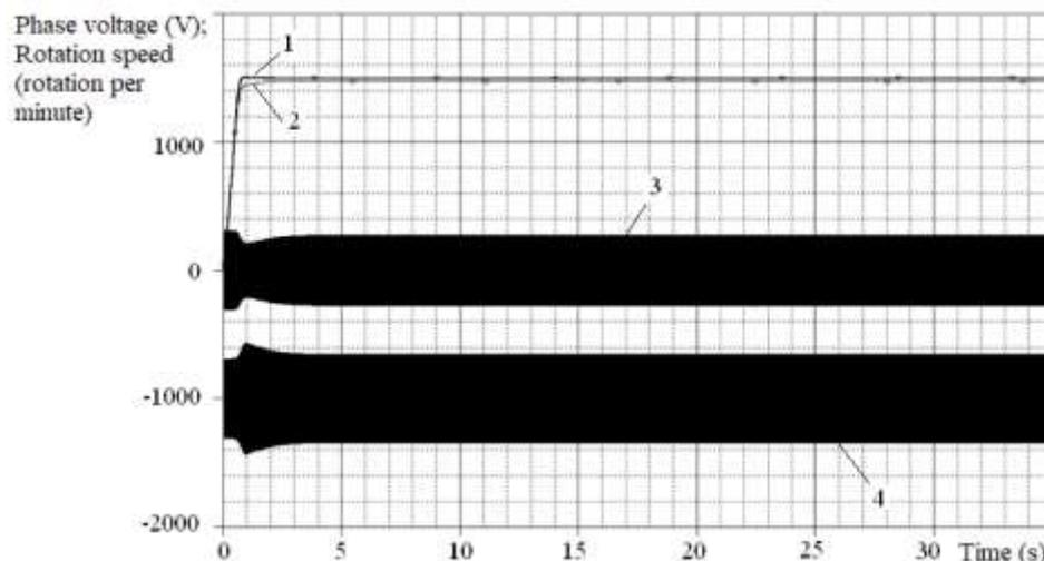
Fig. 5: Results of computer simulation the operation of two NVA-55 with different parameters at the rated supply voltage with the same fan loads on the shafts (graphs of phase voltages and motor rotation speeds). All designations similar to Figure 4
