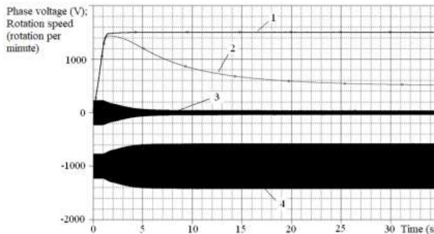
Fig. 4: Results of computer simulation the operation of two series-connected IMs at a supply voltage 25% less than the rated (graphs of phase voltages and IM rotation speeds). 1 – rotation speed of the IM with standard parameters; 2 – rotation speed of the IM with a less main inductance; 3 – graph of the voltage of the IM with a less main inductance. The graph 4 of the IM voltage with standard parameters is shifted down 1000 V for greater clarity
