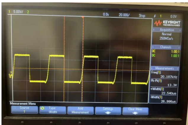
Fig. 17: Supply voltage for DC motor at 50% speed
