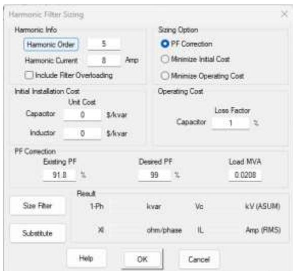
Fig. 6: Harmonic filter sizing done with ETAP for the MCC filter
