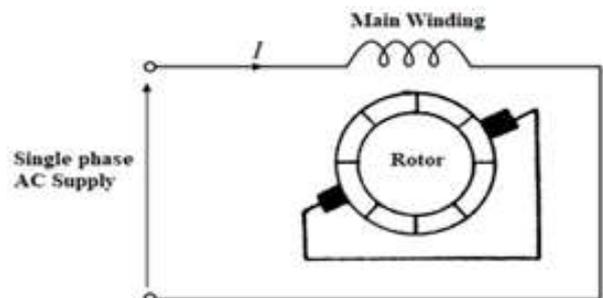
Fig. 5: Repulsion Induction motor (RIM)
