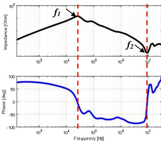
Fig. 8: Impedance and phase angle of PCIM
