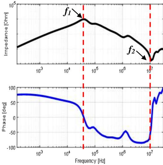
Fig. 7: Impedance and phase angle of CSIM
