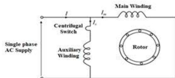
Fig. 2: Split-phase Induction Motor (SPIM)
