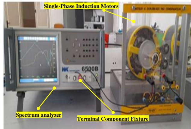
Fig. 6: Experimental setup for differential-mode impedance measurements.
