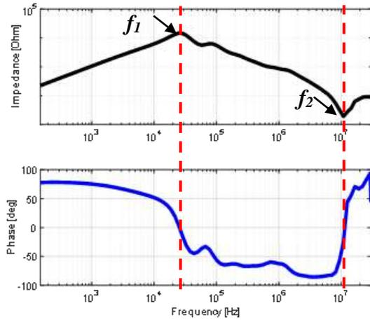
Fig. 9: Impedance and phase angle of SPIM
