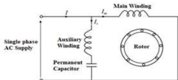
Fig. 4: Permanent Capacitor Induction Motor (PCIM)
