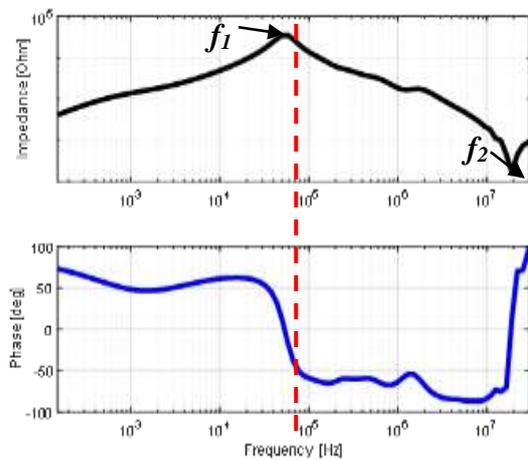
Fig. 10: Impedance and phase angle of RIM
