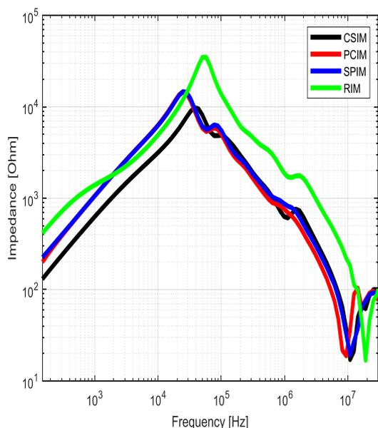
Fig. 11: Impedances comparison of the four motors
