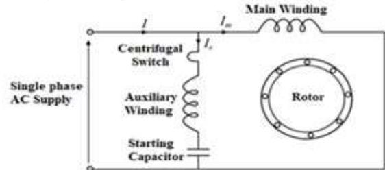
Fig. 3: Capacitor Start Induction Motor (CSIM)
