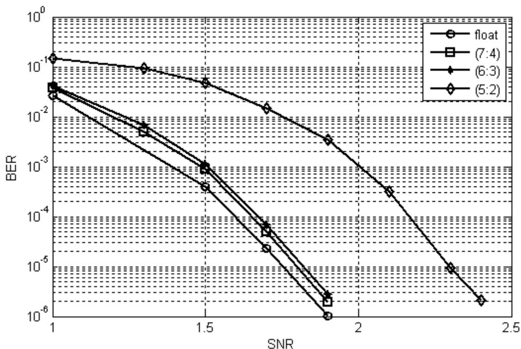
Figure 1. BER Curves of  $LLR_j$  under Layered Offset Min-Sum Algorithm with Different Quantization scheme.
