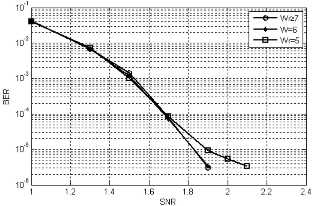
Figure 3. BER Curves of  $r_{ij}$  under Layered Offset Min-Sum Algorithm with Different Quantization
