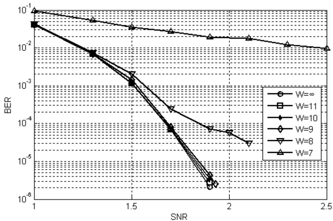
Figure 2. BER Curves of  $Q_j$  under Layered Offset Min-Sum Algorithm with Different Quantization
