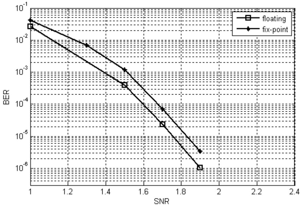
Figure 6. BER Curves of  $Q_j$  under Layered Offset Min-Sum Algorithm with Different Quantization
