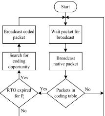
Fig.7. Broadcasting native/coded packet process
