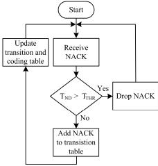
Fig.6. Handling NACK packets process
