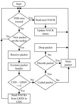
Fig.5. Signalization and decoding processes
