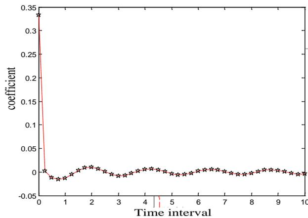
Fig 4 Auto correlation function of 3D degenerate 2D channel model when UAV stop
