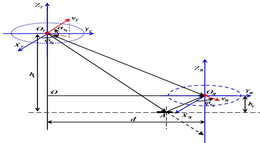
Fig 2 line-of-sight and specular reflecting component
