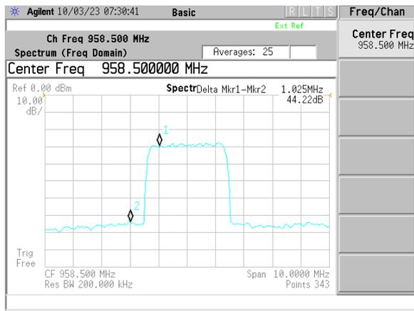
Fig. 4a. The measured power spectra of the LTE R9 3 MHz 16 QAM signal at the input of the reconfigurable filter without I/Q imbalance.
