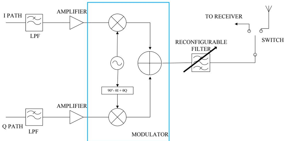
Fig. 1. Wireless transmitter with undesired effects
