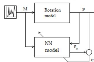
Fig. 5 The block diagram of neural identification
