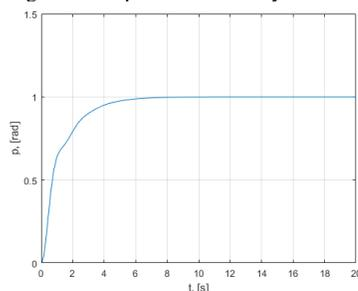
Fig. 2 The step response of the position control system.
