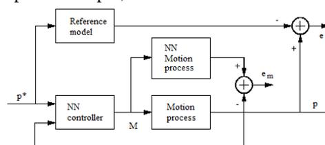
Fig. 4 Neural model reference control structure
