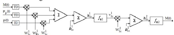
Fig. 7 The bloc diagram of the structure of the neural controller
