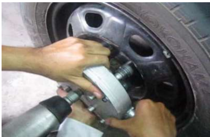
Fig. 3 Removing all wheel nuts using VAWNR and impact wrench
