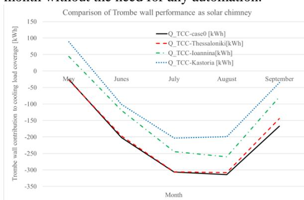
Figure 13. Comparison of Trombe wall performance as solar chimney in examined locations
