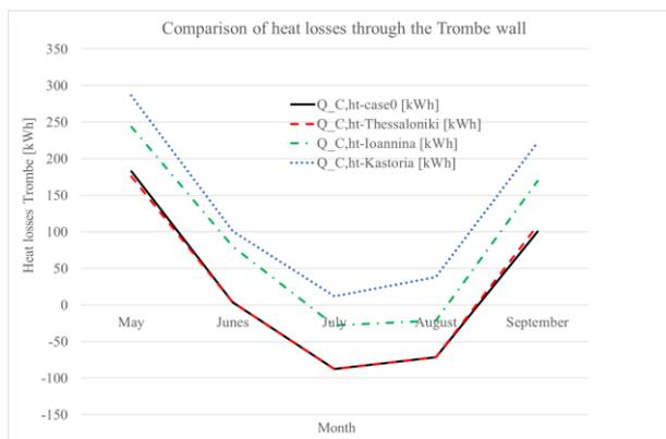
Figure 12. Heat losses through Trombe wall in the examined locations
