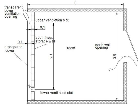
Figure 3. Cross-section for the solar chimney operation
