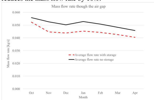
Figure 4. Mass flow rate through the air gap
