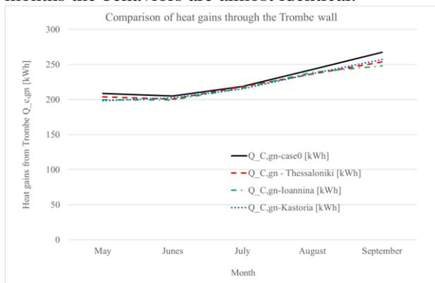
Figure 11. Heat gains from the Trombe in the examined locations
