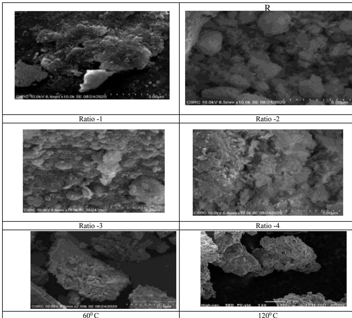
Fig. 5: A mix of red-based geopolymer bricks cured at 600 C and 1200 C shows different alkali activator ratios
