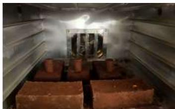
Fig. 1: Red mud-based Geopolymer Bricks
