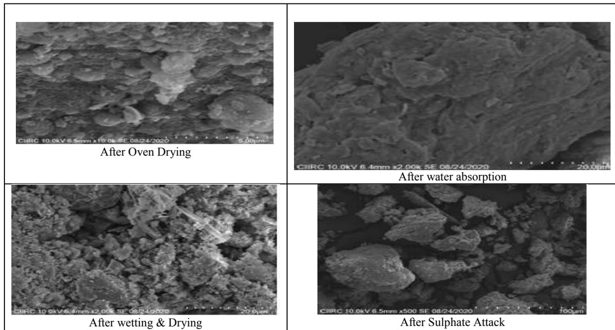
Fig. 6: SEM image of brick of 60:10:30 mix proportion at 1: 2.5 alkali activator ratio subjected to various conditions
