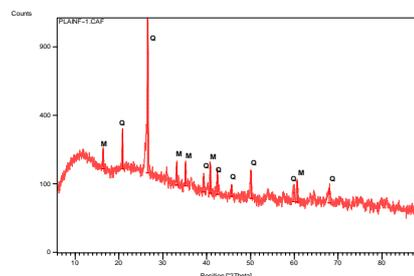
Fig. 3: XRD image of Fly Ash
