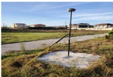
Fig. 5: Global Positioning Passive State Network Point, First Order
