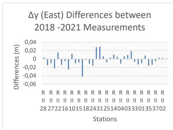
Fig. 9: The changes of coordinates  $\Delta y$ , (Y=East) between 2018-2021 Measurements
