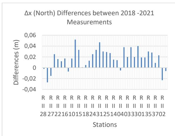
Fig. 8: The changes of coordinates  $\Delta x$ , (X=North) between 2018-2021 Measurements
