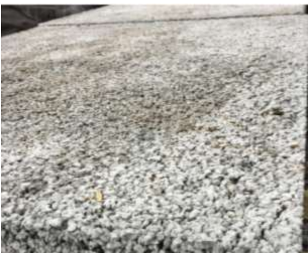
Fig. 9: Water permeable concretes
