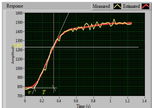
Fig. 8 DC Motor open loop identification of the transfer function
