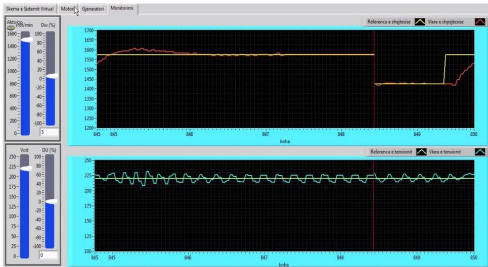
Fig. 21 SG 8241 step responses for 10% increment of DC Motor 8211 speed set-point
