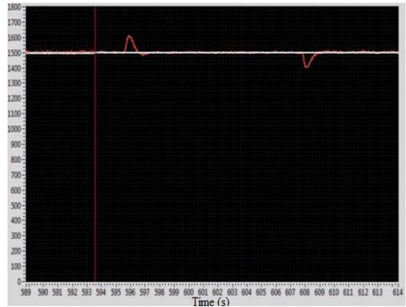
Fig. 18 SG field voltage changes influence to the speed control loop
