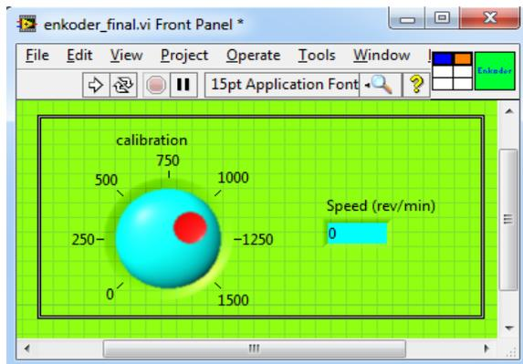
Fig. 3 Front Panel of speed measuring virtual instrument
