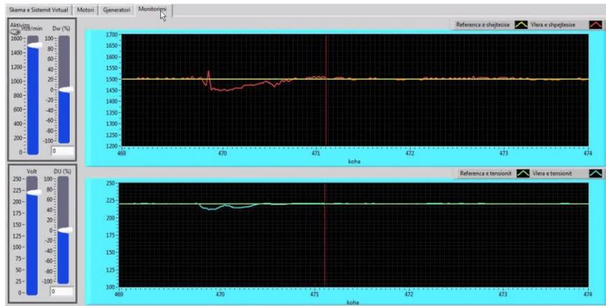
Fig. 24 SG 8241 step responses when the three-phase resistive load increase from 0,3 p.u. to 0,6 p.u.
