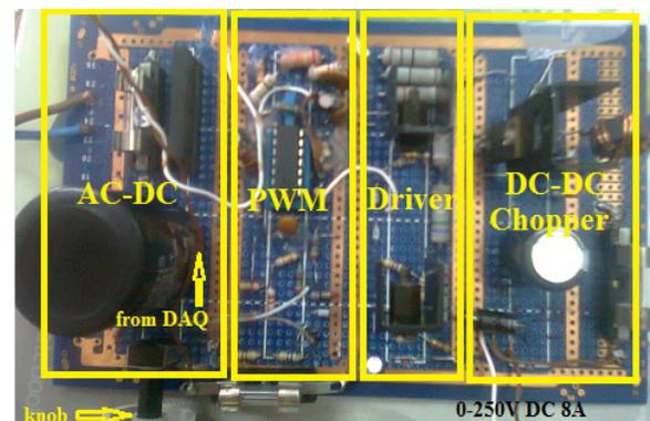
Fig. 4 Custom-built AC-DC converter
