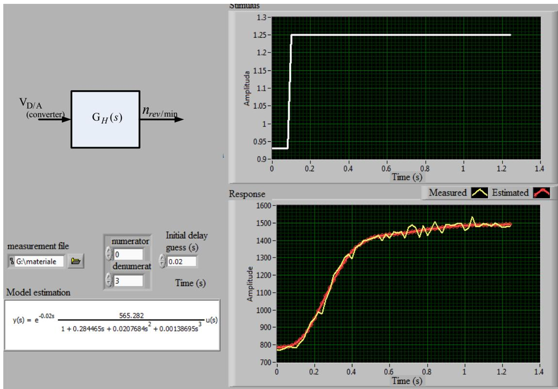
Fig. 7 Front Panel of the instrument for DC Motor mathematical model identification in LABVIEW
