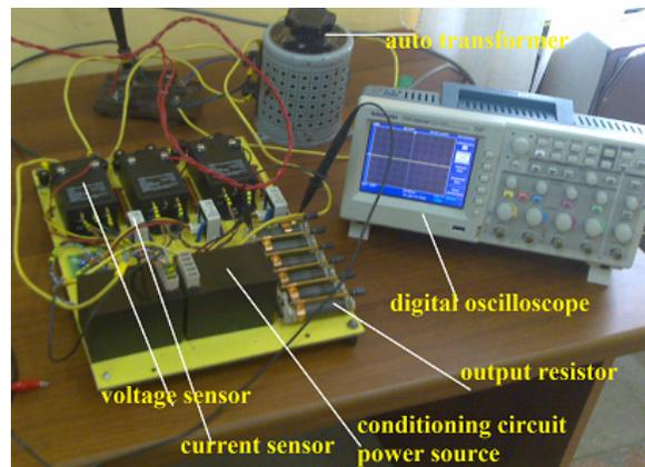
Fig. 2 Three-phase electrical quantities measurement module
