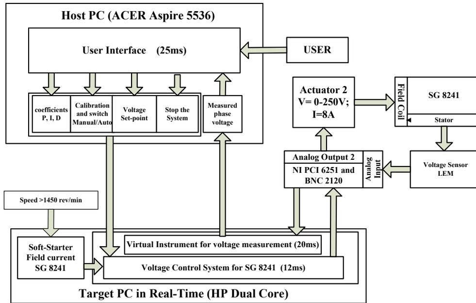
Fig. 12 Functional block diagram of the Voltage Control and Monitoring System
