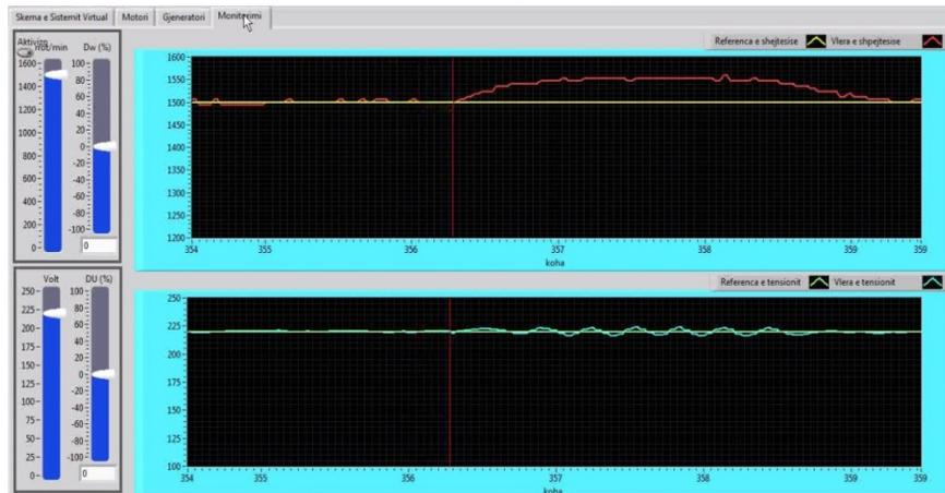
Fig. 23 SG 8241 step responses when the three-phase resistive load decrease from 1 p.u. to 0,6 p.u.
