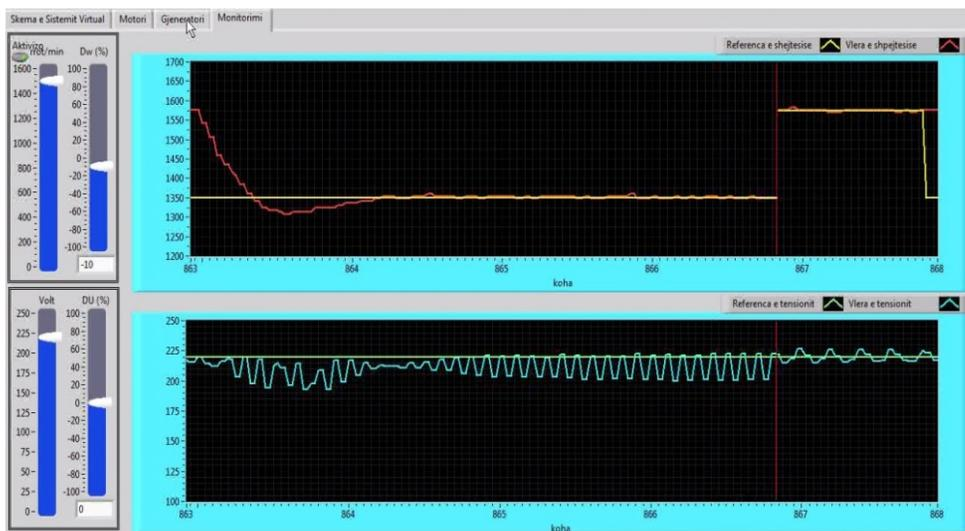
Fig. 22 SG 8241 step responses for 15% decrement of DC Motor 8211 speed set-point
