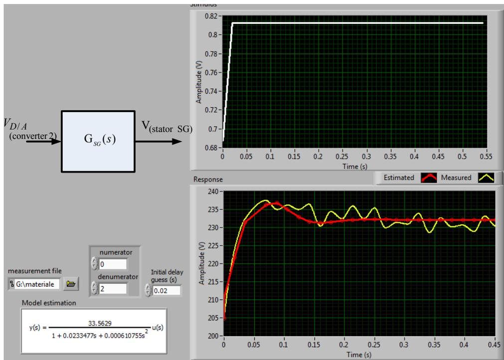
Fig. 9 Front Panel of the instrument for SG mathematical model identification in LabVIEW
