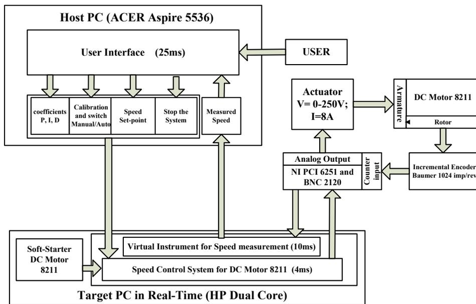
Fig. 11 Functional block diagram of the Speed Control and Monitoring System
