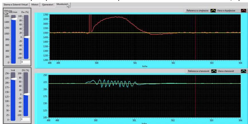
Fig. 25 SG 8241 step responses when the three-phase resistive load decrease from 1 p.u. to 0 p.u.
