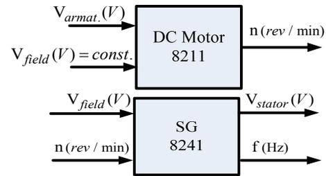
Fig. 6 DC Motor and SG blocks with the inputs and outputs for controlling and monitoring
