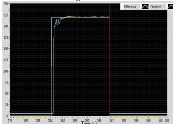
Fig. 17 SG voltage control response for +100% step (0V to 220V) in the voltage set-point
