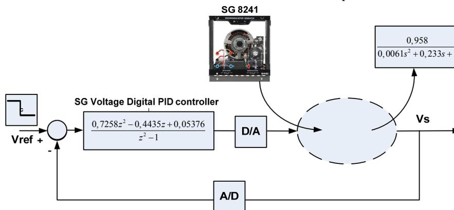
Fig. 15 SG 8241 voltage control closed loop using HIL
