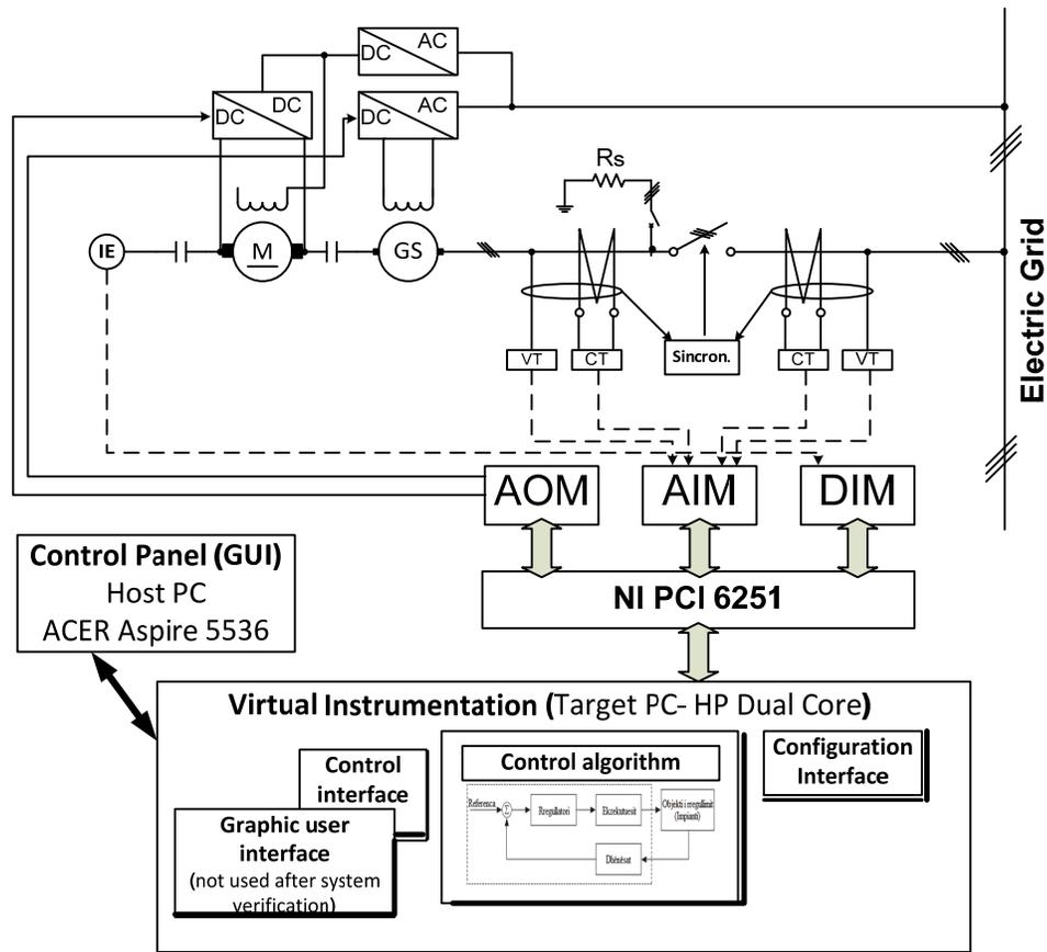
Fig. 1 Overall block diagram of the synchronous generator control and monitoring system in LabVIEW
