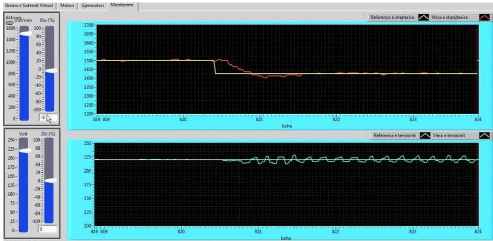
Fig. 20 SG 8241 step responses for 5% decrement of DC Motor 8211 speed set-point
