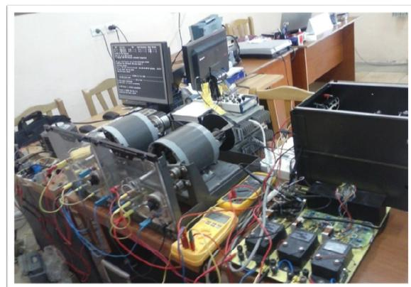
Fig. 14 SG bench during Virtual System experimental verification
