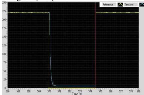
Fig. 16 SG voltage control response for -100% step (220V to 0V) in the voltage set-point
