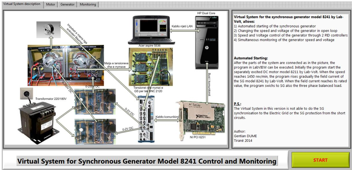
Fig. 13 Front Panel of the Virtual System for SG 8241 control and monitoring
