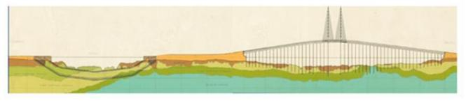
Fig. 5 A typical longwise profile form Cobenhagen to Malmoe in alignment (Light brown = fill, brown = glacial deposits & green, yellow, green = Upper, Middle and Lower Copenhagen limestone Units, blue = Bryozoan limestone) [18]
