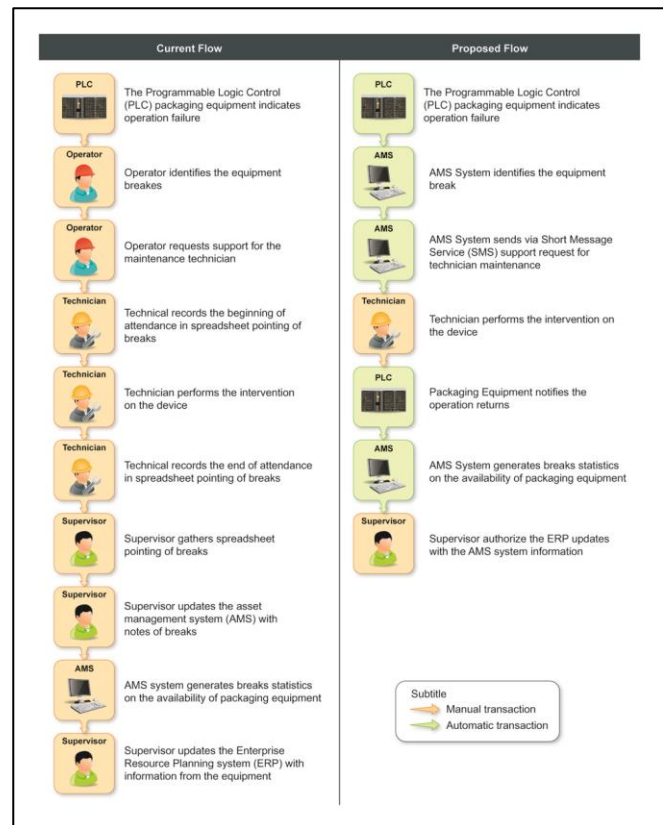
Fig. 3: Flow of current and proposed corrective maintenance in packaging equipment
