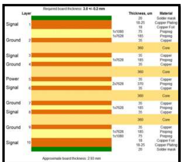
Fig. 1: Sample of 10-layer firm stack-up guaranteeing the power integrity in IoT/mobile device LP-PCB design for LPES.
