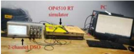
Fig. 14: OPAL4510-RT Simulator test bench
