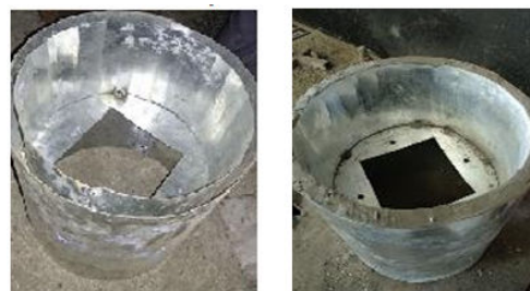
Fig. 7. manufacturing of skirt for stove
