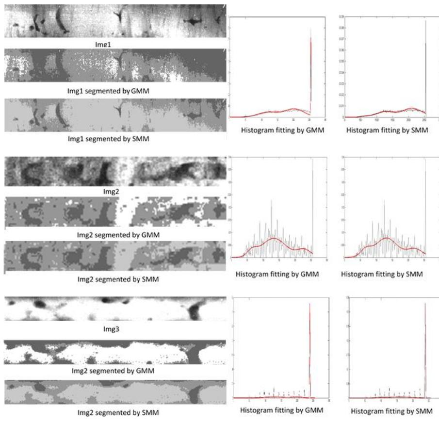
**Fig. 2.** Industrial radiography images segmented by GMM and SMM, Histogram fitting by GMM and SMM,
