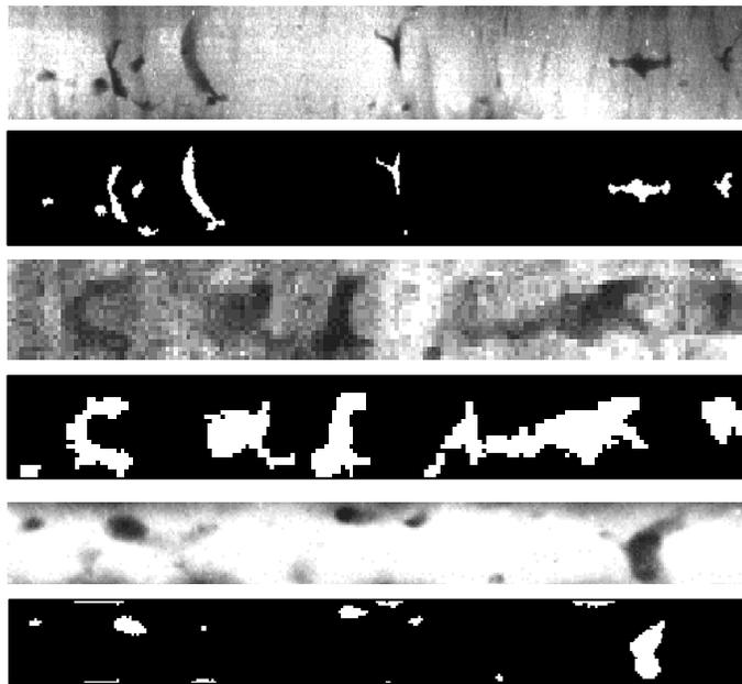
**Fig. 1.** Radiographic images and the corresponding hand segmented Images (Reference Images)
