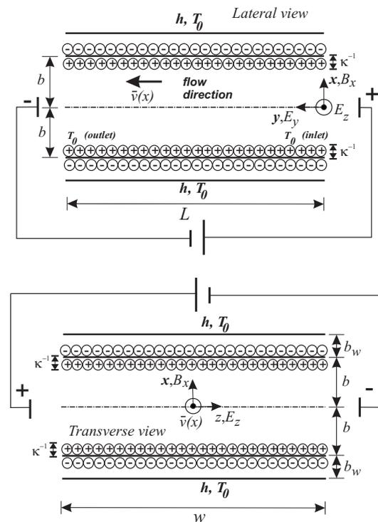
Fig. 1. Electroosmotic and magnetohydrodynamic flows in a parallel flat plates microchannel.
