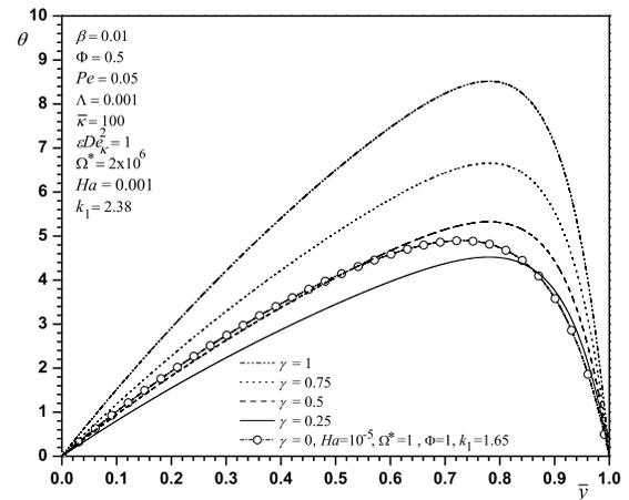
Fig. 2. Dimensionless temperature distribution as function of the dimensionless axial coordinate in combined electroosmotic and magnetohydrodynamic flows with different values of the parameter  $\gamma$ .
