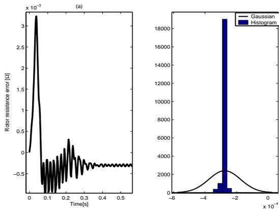
Figure 8: (a) stator resistance error. (b) Gaussian and histogram of error rotor resistance.
