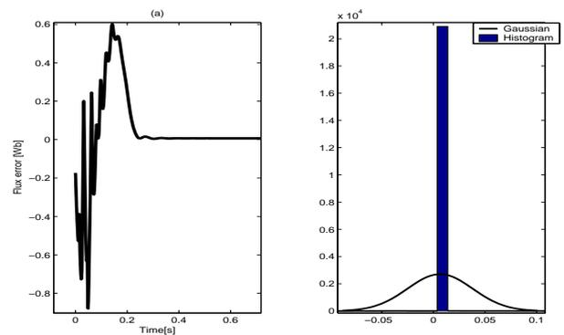
Figure 5: (a) Flux error. (b) Gaussian and histogram of error flux.
