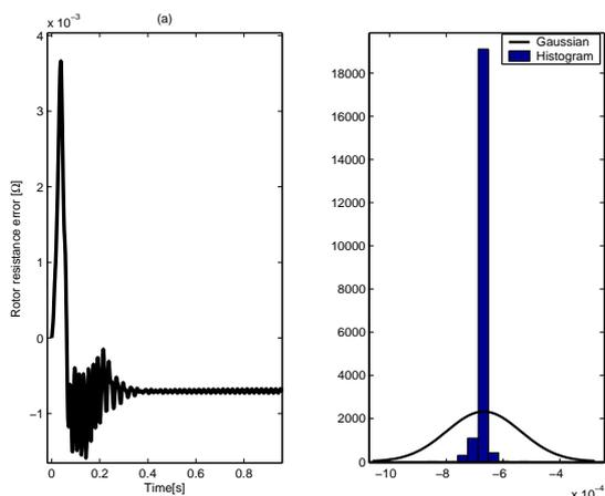
Figure 12: (a) stator resistance error. (b) Gaussian and histogram of error rotor resistance.
