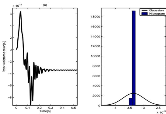
Figure 4: (a) stator resistance error. (b) Gaussian and histogram of error rotor resistance.
