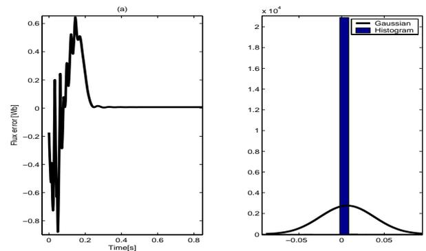
Figure 9: (a) Flux error. (b) Gaussian and histogram of error flux.
