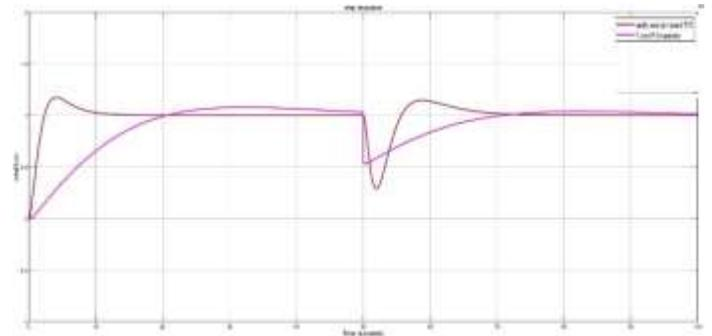
Fig. 2 Step response of DC motor
