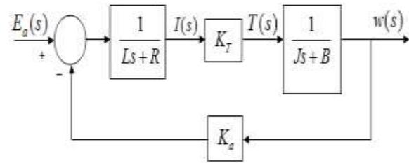
Fig 1: Block diagram of a current-controlled DC motor
