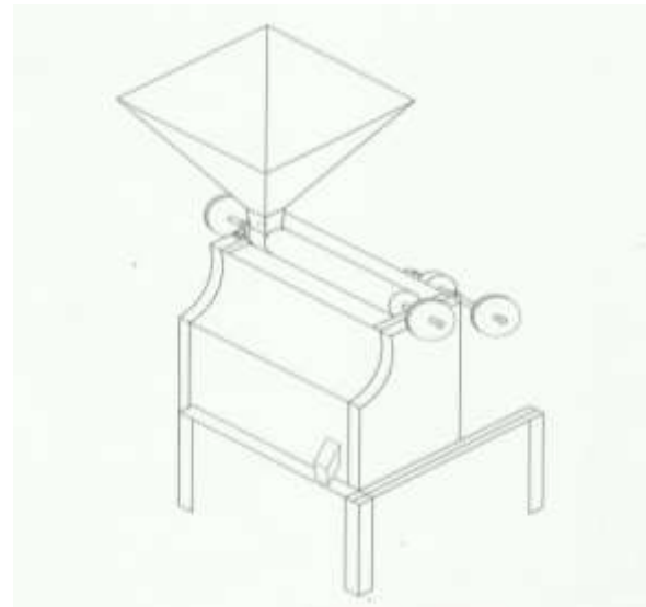
Fig. 3: Schematic representation of the rice milling machine
