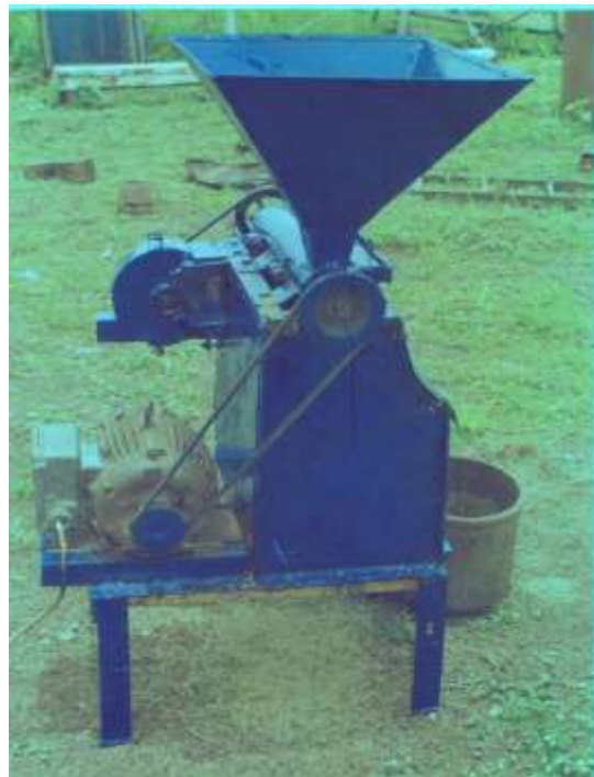
Fig. 1: Pictorial side view of the rice milling machine
