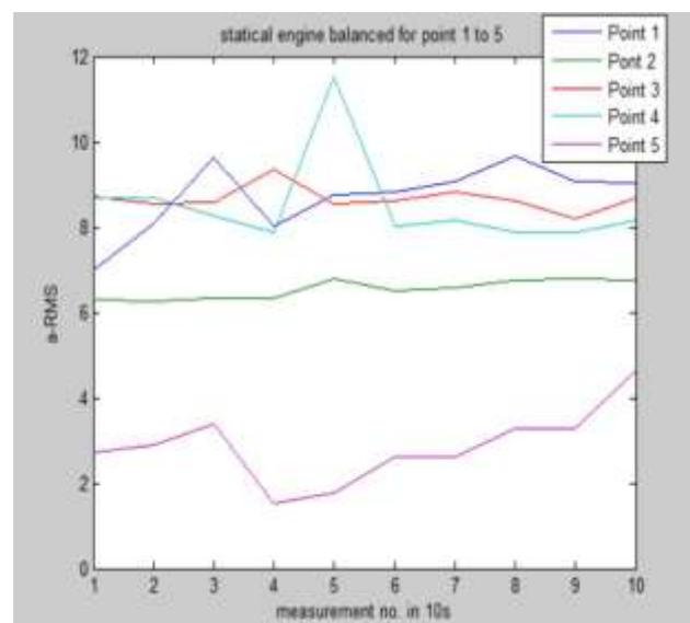
Fig. 8: RMS accelerations [mm/s<sup>2</sup>] of a static balanced engine (Point 1 to Point 5).
