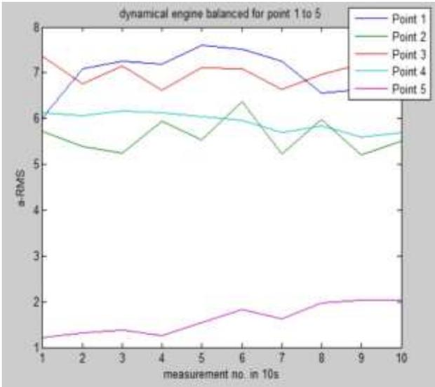
Fig. 9: RMS accelerations [mm/s<sup>2</sup>] of a dynamic balanced engine (Point 1 to Point 5).
