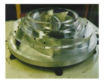
Fig.2 SHF Impeller with transparent
