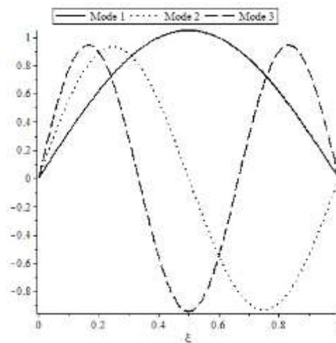
Fig. 4: The first, second and third mode shapes
