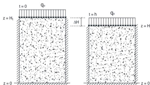
Figure 1. Physical scheme of 1D consolidation
