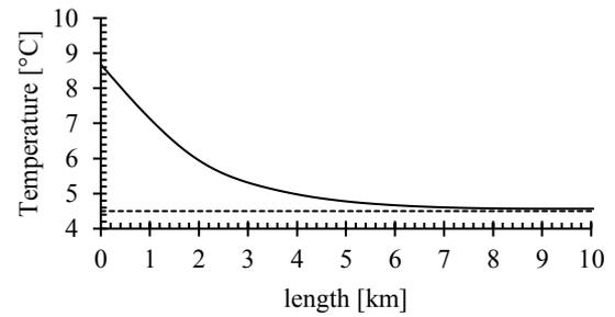
Fig. 1: Temperature variation along the CWP, with the dotted line marking the  $4.4^\circ\text{C}$  seawater temperature at 1 km depth
