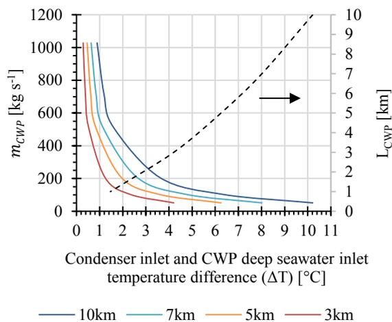
Fig. 2: Temperature difference between condenser inlet and CWP deep seawater inlet ( $\Delta T$ ) for different mass flow rates and CWP lengths
