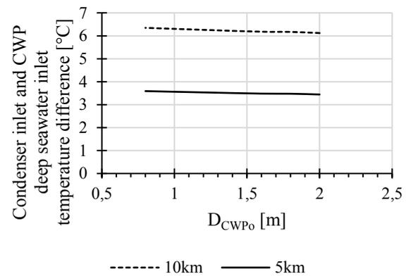
Fig. 3: CWP diameter versus the temperature difference between the condenser inlet and the CWP deep seawater inlet ( $\Delta T$ ), for two different CWP lengths of, 10km and 5km
