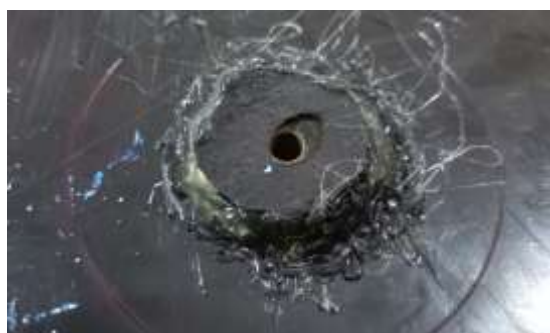
Figure 2. The Cover of the Plastic Container's Cover after a Hole was Punched through it
