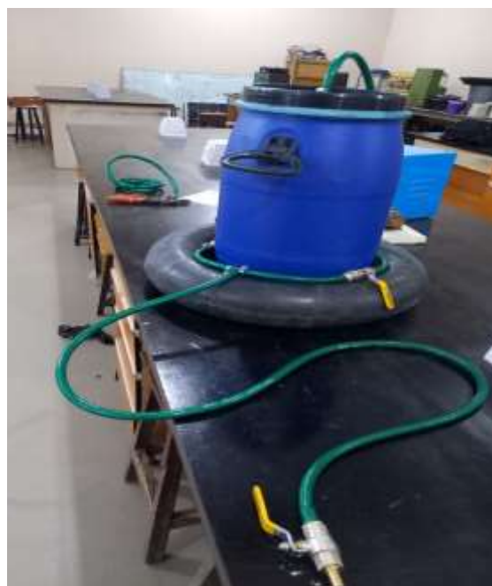
Figure 10. Barrel Drum Biogas Digester
