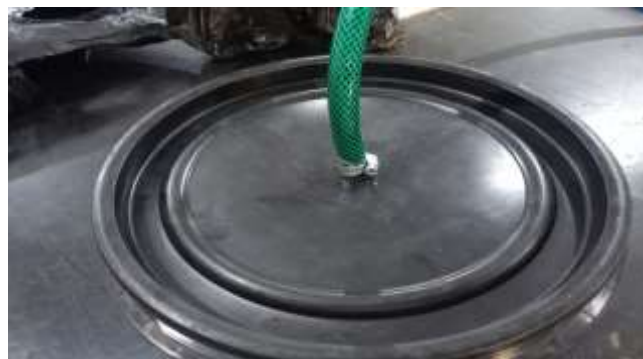
Figure 4. The Biogas Digester Terminated Rubber Hose with Clip
