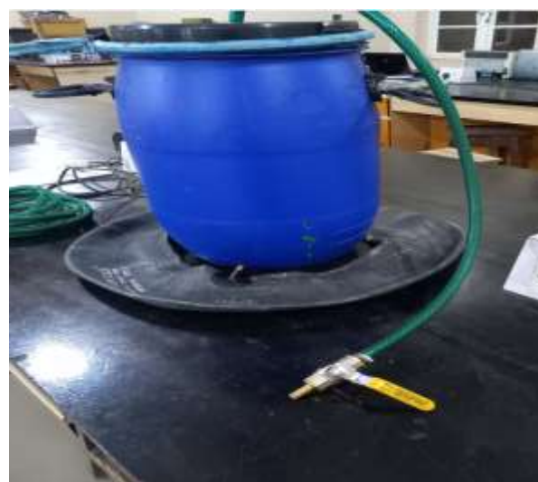
Figure 5. The Gas Tap Termination from the Fab Connected to the Cover of the Biogas Plastic
