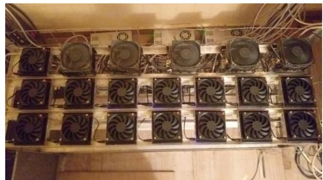
Fig. 3: The utilized Odroid single-board computers (15x Odroid-N2+ and 5x Odroid-MC1)
