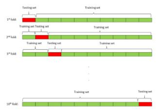
Fig. 3: An Illustration of the 10 fold cross-validation
