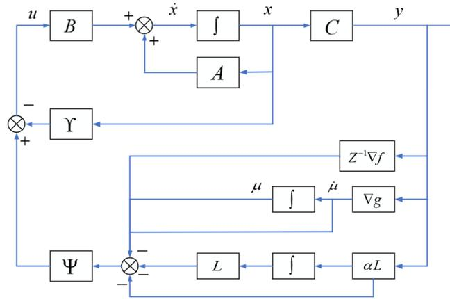
Figure 1: The controller to solve the optimization problem (3).
