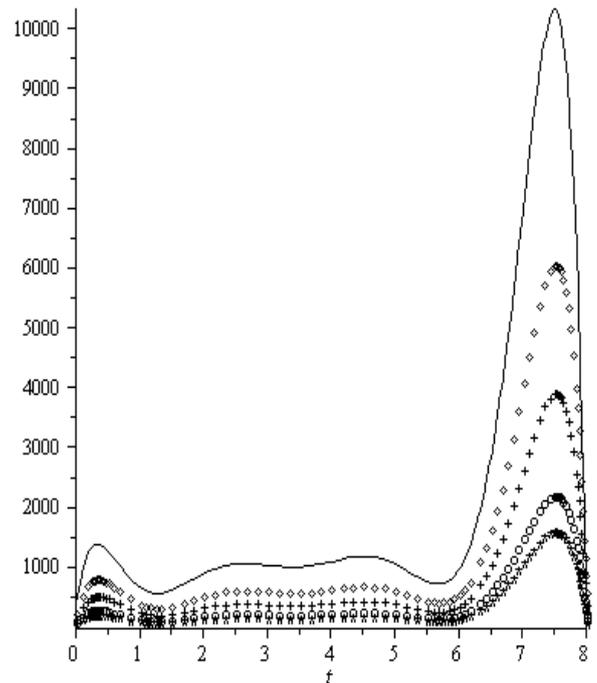
Fig. 16. The dependence  $S_\sigma(C, \lambda)$ , obtained for different varies of the Poisson's ratio. The solid curve corresponds to  $\sigma=0.1$  (concrete), quadrangles -  $\sigma=0.2$  (cast iron), crosses -  $\sigma=0.3$  (cuprum), circles -  $\sigma=0.4$  (plumbum), asterisks -  $\sigma=0.45$  (cautchouc). The initial condition for function  $y(x)$  here  $y'(0)=0.5$ .
