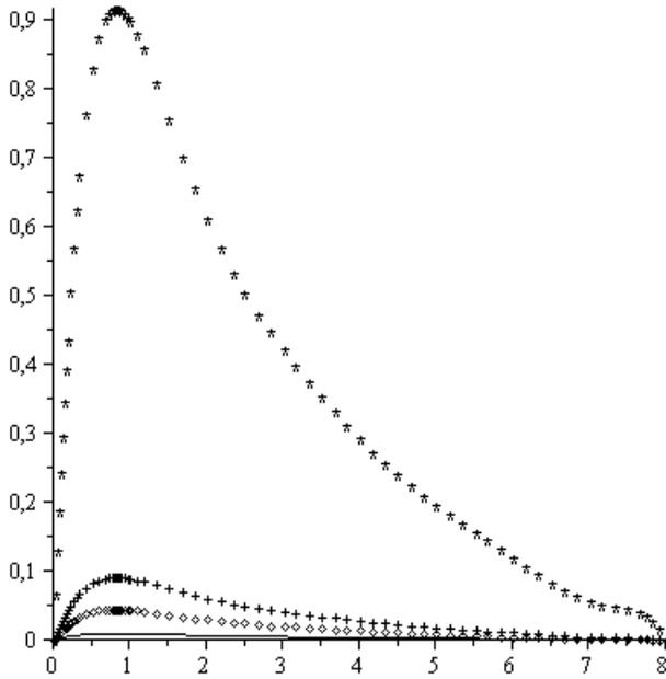
Fig.4. The function  $y(x)$ , obtained at a fixed value of the Poisson's ratio  $\sigma = 0.45$  and at different initial conditions. The solid curve, enlarged tenfold, corresponds to  $y'(0) = 0.01$ , quadrangles -  $y'(0) = 0.5$ , crosses -  $y'(0) = 1$ , asterisks -  $y'(0) = 10$ .
