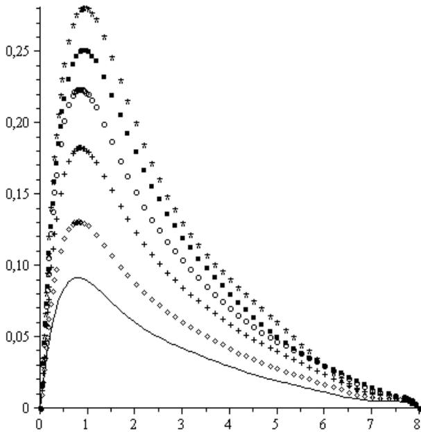
Fig.1. The function  $y(x)$ , obtained for the fixed initial condition  $y'(0)=1$  and at different coefficient values of the Poisson's ratio  $\sigma$ . All the curves are in accord with theoretical meanings of Poisson's coefficient (from now on). Solid curve conforms with  $\sigma = 0.45$ , quadrangles -  $\sigma = 0.4$ , crosses-  $\sigma = 0.3$ , circles -  $\sigma = 0.2$ , black boxes -  $\sigma = 0.1$ , asterisks-  $\sigma = 0.01$ .
