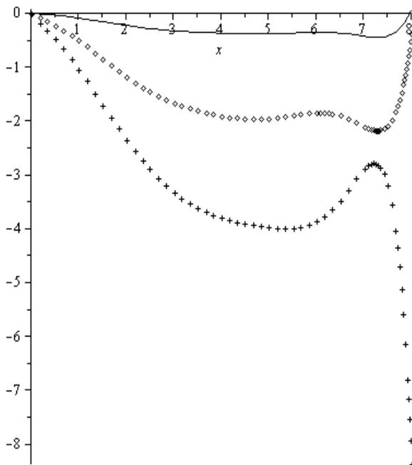
Fig.11. The dependence  $u_z(x)$ , constructed under constant value of the Poisson's ratio  $\sigma = 0.2$  for different initial conditions. The solid curve, enlarged tenfold corresponds to  $y'(0) = 0.01$ , circles -  $y'(0) = 0.5$ , crosses -  $y'(0) = 1$ .
