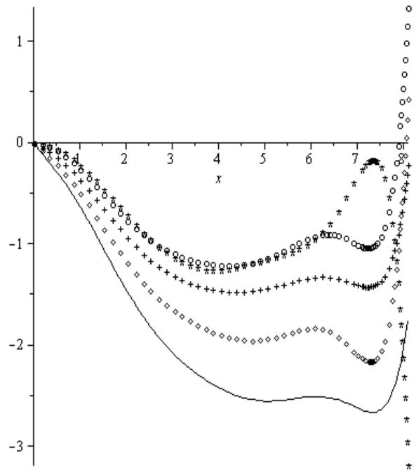
Fig.8. The dependence  $u_z(x)$ , constructed under a constant condition  $y'(0)=0.5$  for the different values of the Poisson's ratio  $\sigma$ . The solid curve corresponds to  $\sigma=0.1$ , quadrangles -  $\sigma=0.2$ , crosses -  $\sigma=0.3$ , circles -  $\sigma=0.4$ , asterisks -  $\sigma=0.45$ .
