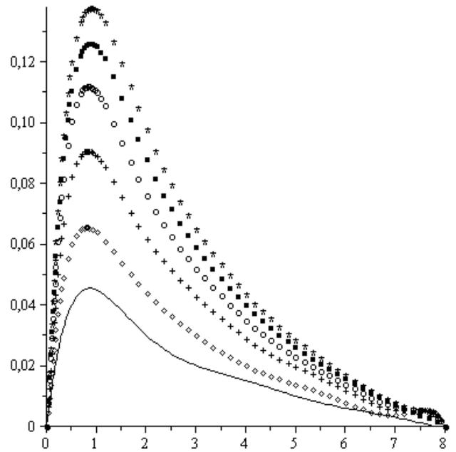
Fig.2. The function  $y(x)$ , obtained for an fixed initial condition  $y'(0)=0.5$  and at different coefficient values of the Poisson's ratio  $\sigma$ . Solid curve conforms with  $\sigma = 0.45$ , quadrangles -  $\sigma = 0.4$ , crosses -  $\sigma = 0.3$ , circles -  $\sigma = 0.2$ , black boxes -  $\sigma = 0.1$ , asterisks -  $\sigma = 0.01$ .
