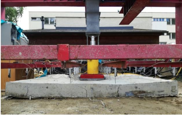
Fig. 1 - (Typical concrete slab with dimensions 2 x 2 m during testing. Author: Z.N.
