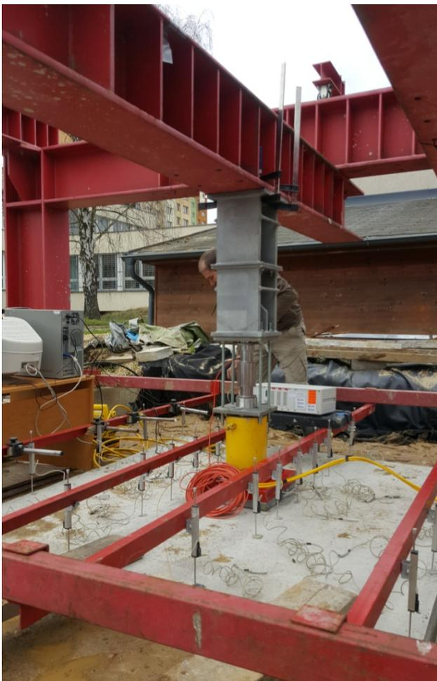
Fig. 2 - Photo of the testing device. Author: Z.N.
