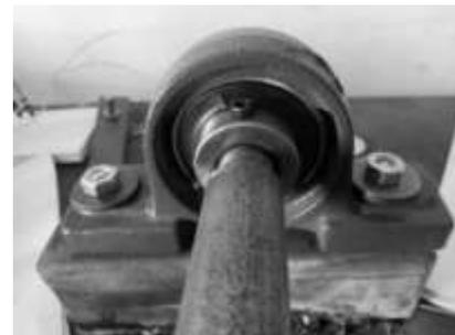
Fig. 38: Bearing with holder bolted to frame
