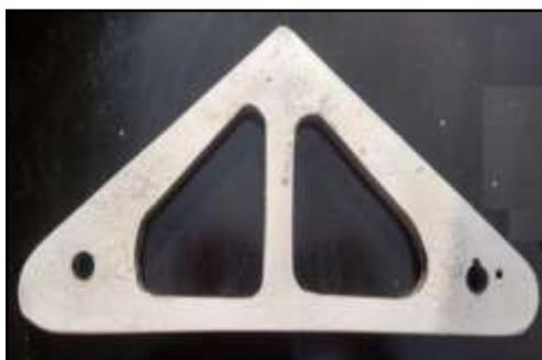
Fig. 36: Fabricated linkages (rocker)
