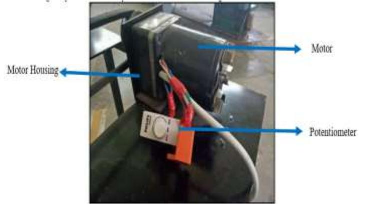
Fig. 42: Motor with potentiometer
