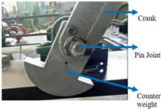
Fig. 40: Crank and counterweight
