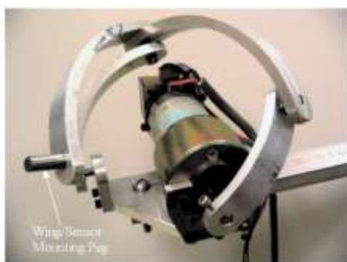
Fig. 14: Spherical Four-bar Mechanism for flapping in Micro-air vehicle [17]
