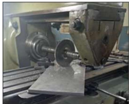
Fig. 32: Cutting of coupler on horizontal milling machine
