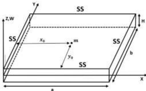
Fig. 1: A simply supported plate with an added mass at  $(x_0, y_0)$
