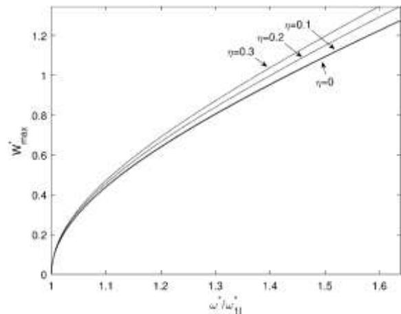
Fig. 4: the backbone curve of a plate  $\alpha = 0.6$  carrying an added mass at (0.25, 0.5)
