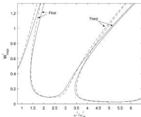
Fig. 6: The frequency response of a plate  $\alpha = 0.6$  subjected to a harmonic concentrated force  $F = 1N$  applied at the plate center. The continuous line presents the frequency response of a simply supported plate with no added mass. The discrete line presents the frequency response of a simply supported plate carrying an added centric mass with added mass ratio  $\eta = 0.1$
