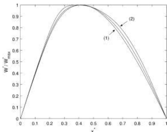
Fig. 5: Comparison of the first mode shape in large amplitude of a simply supported rectangular plate  $\alpha = 0.6$  carrying an eccentric mass  $\eta = 0.1$  at  $(0.25,0.5)$ , (1) lowest amplitude, (2) highest amplitude
