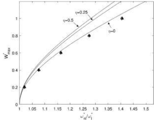
Fig. 2: Presentation of values of Table 2, Table 3, Table 4 in case of  $\alpha = 1$ , results of R. H. Gutiérrez and P. A. A. Laura [10] are presented by symbols: ( $\diamond$ ) in case of without mass, ( $\Delta$ ) for  $\eta = 0.25$  and ( $*$ ) for  $\eta = 0.5$ . The results of the present work are presented by a line
