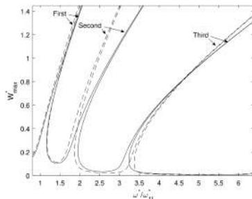
Fig. 8: The frequency response of a plate  $\alpha = 0.6$  subjected to a harmonic concentrated force  $F = 0.3N$  applied at (0.25,0.5). The continuous line presents the frequency response of a simply supported plate with no added mass. The discrete line presents the frequency response of a simply supported plate carrying an added eccentric mass at (0.25,0.5) with added mass ratio  $\eta = 0.1$
