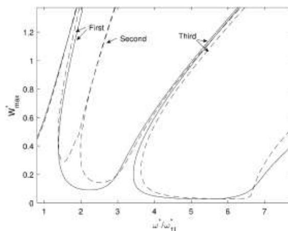
Fig. 7: The frequency response of a plate  $\alpha = 0.6$  subjected to a harmonic concentrated force  $F = 1N$  applied at the plate center. The continuous line presents the frequency response of a simply supported plate with no added mass. The discrete line presents the frequency response of a simply supported plate carrying an added eccentric mass at  $(0.25,0.5)$  with added mass ratio  $\eta = 0.1$
