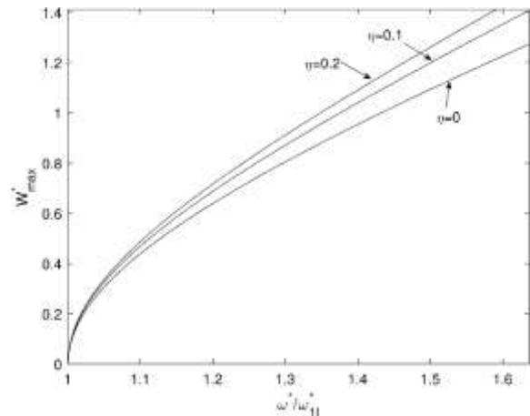
Fig. 3: the backbone curve of a plate  $\alpha = 0.6$  carrying a centric mass
