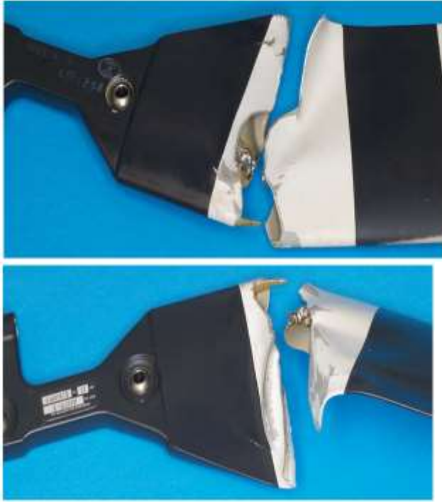
Figure (2) shows models of the main blades of destroyed helicopters, showing the locations and shape of the crack, its growth and collapse of the main blade
