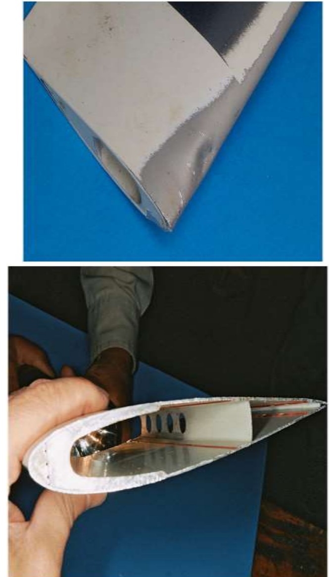
Figure (1) shows sections of the main blade of the helicopter on which the test was conducted
