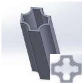
Fig. 3(b): The geometry of the outer wall and spacer grid along with an intent image of the internal view.
