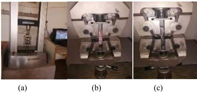
Fig 2: (a) tensile test device, (b) reinforced sample fracture and (c) pure resin sample fracture.
