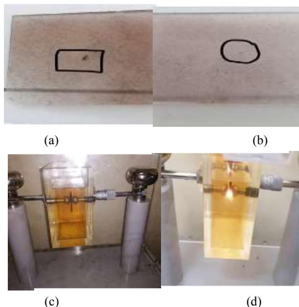
Fig. 6: (a) samples under test; (b) breakdown moment; (c) iron reinforced sample shape after breakdown; (d) pure resin sample shape after breakdown
