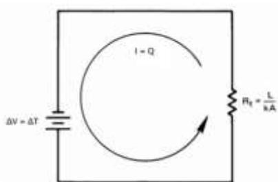
Fig. 5: Ohms law analogy to conduction through a slab
