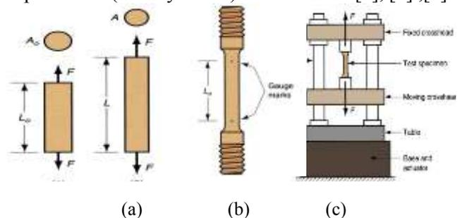
Fig. 1: Tensile test (a) Tensile force applied in (1) and (2), resulting in the elongation of the material, (b) Typical test specimen and (c) Setup of the tensile test
