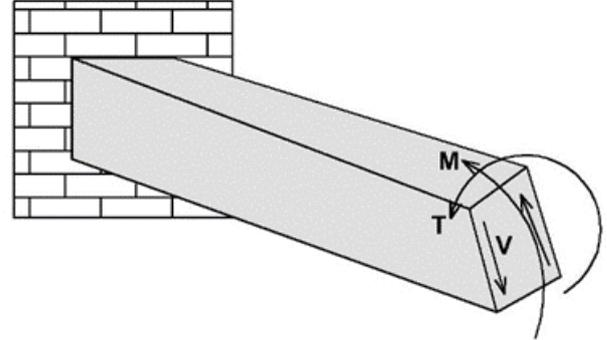
Fig. 5: Loads acting on the beam section
