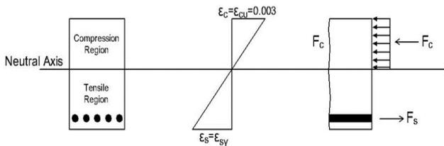
Fig. 4: Internal forced forming in the beam cross-section
