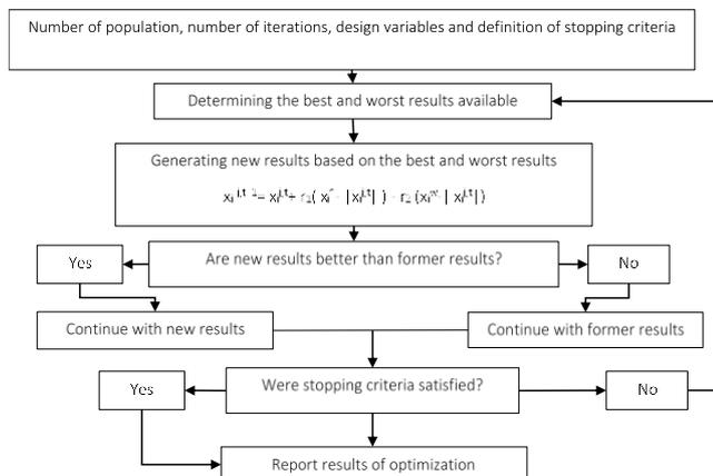
Fig. 1: Flow chart of the optimization method
