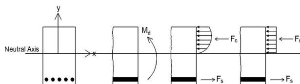
Fig. 3: Actual load distribution and equivalent load distribution in the compression zone
