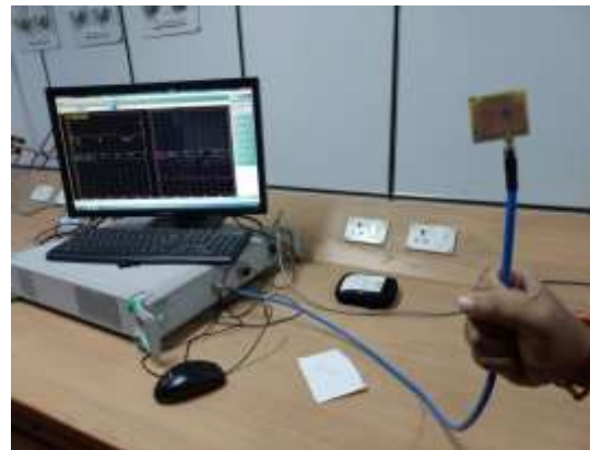
Figure 3.38: VNA testing of the antenna in free space
