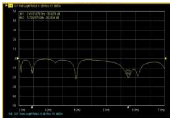
Fig.4.2: Measured return loss S11(dB) of proposed antenna in free space
