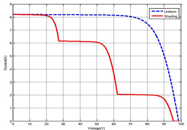
Fig. 9 Comparison between I-V curve uniform and partially shaded PV array .
