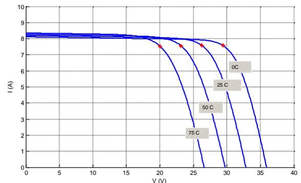
Fig. 5 Current VS Voltage Characteristic curve (G=1000W/m²)
