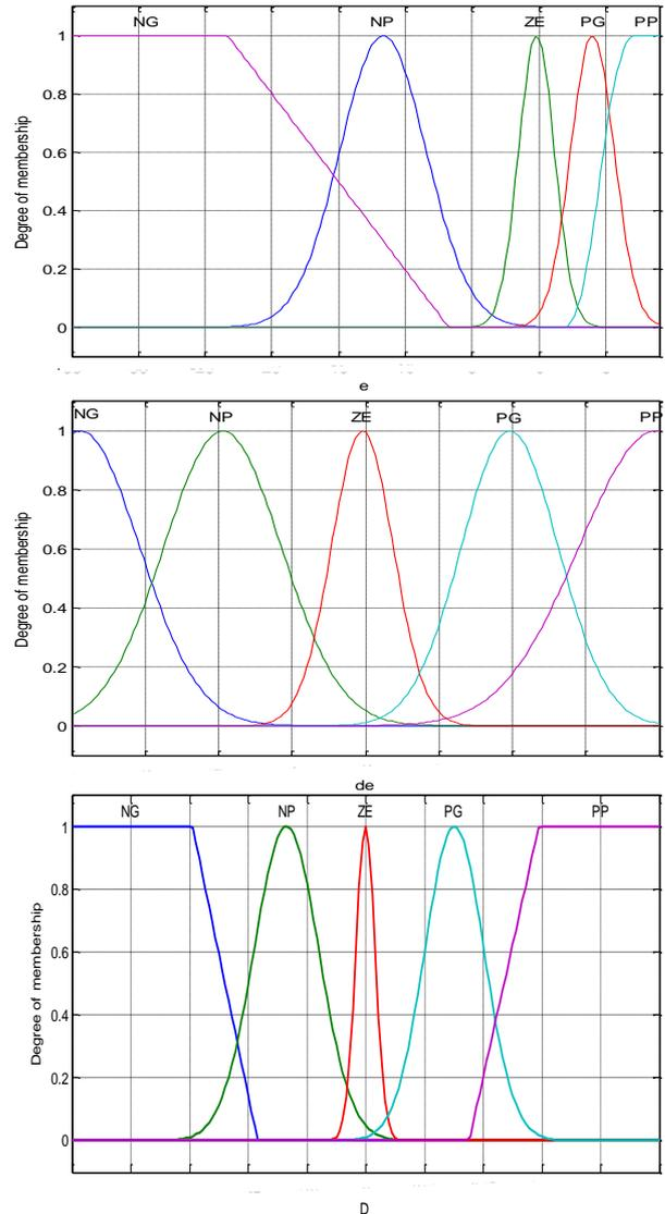
Fig. 14 Fuzzy logic membership functions for inputs and output variables
