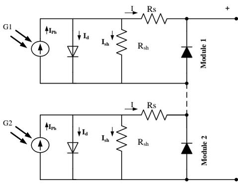
Fig. 7 Circuit diagram of partial shaded modules.
