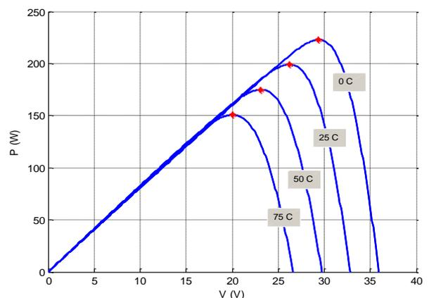
Fig. 6 Power VS Voltage Characteristic curve (G=1000W/m<sup>2</sup>)
