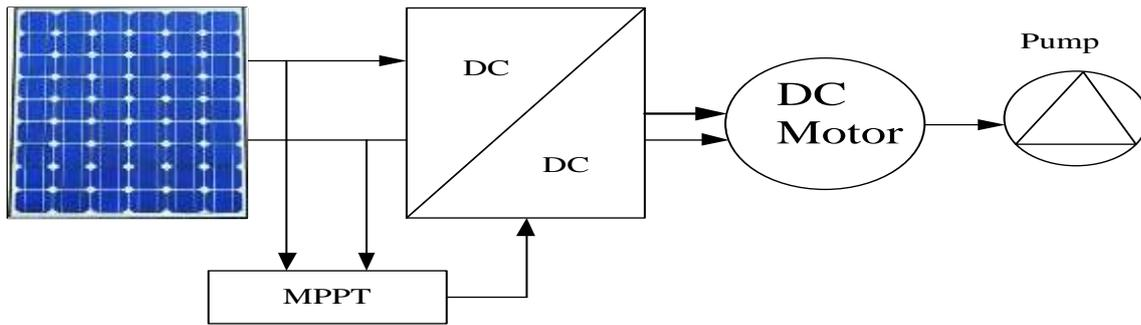
Fig. 15 Block diagram of the D.C water pump
