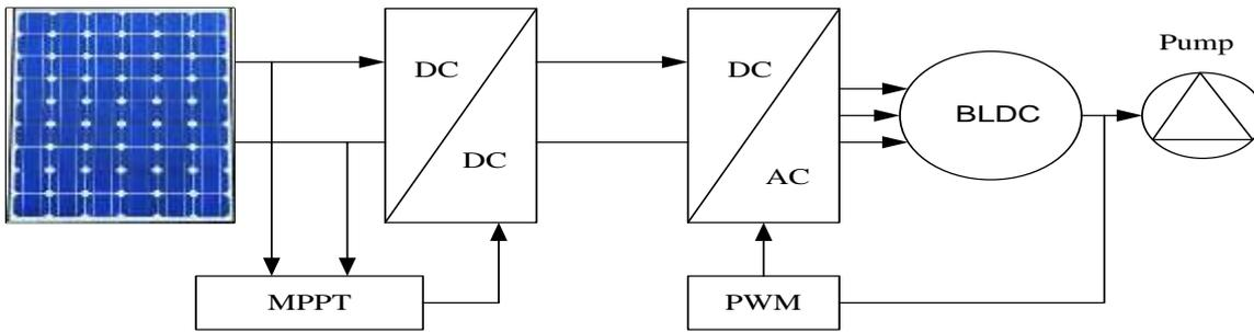
Fig. 1 Block diagram of the BLDC water pumping system
