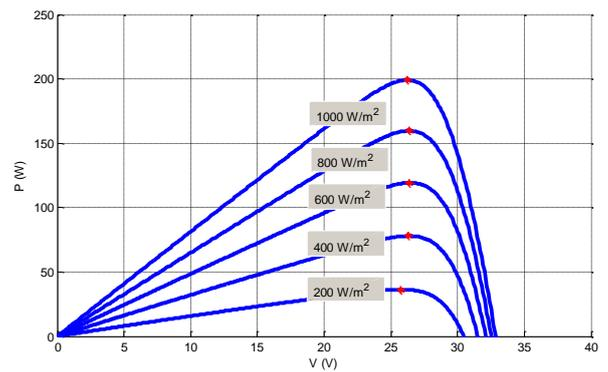
Fig. 4 Power VS Voltage Characteristic curve (T=25°C)
