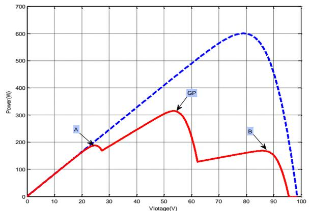
Fig. 10 Comparison between P-V curve uniform and partially shaded PV array
