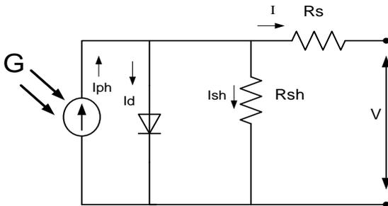
Fig. 2 Block of equivalent circuit of PV cell
