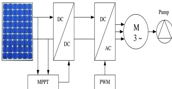
Fig. 16 Block diagram of the A.C water pumping system
