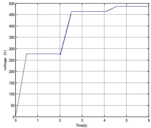
Fig. 18 boost converter output voltage
