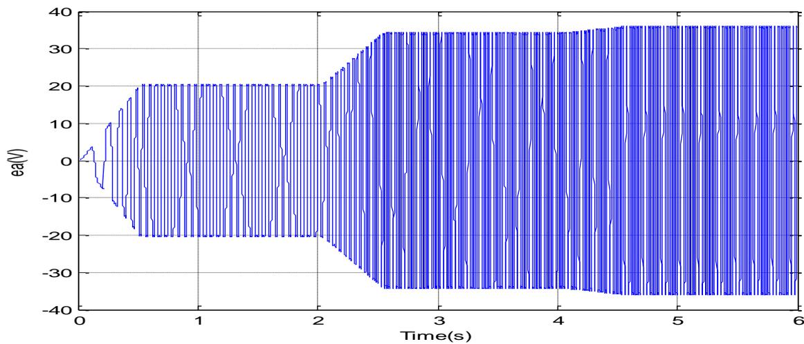
Fig.22 Stator back EMF e\_a (V)
