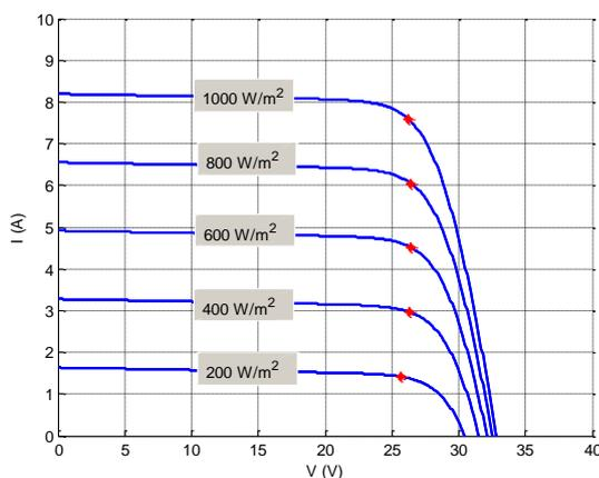
Fig. 3 Current VS Voltage Characteristic (T=25°C)
