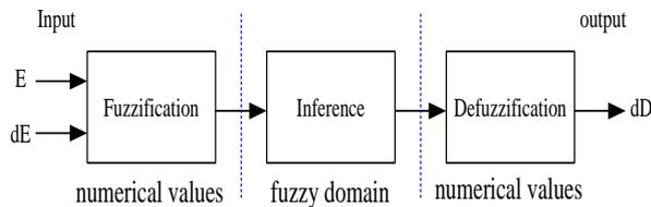
Fig. 13 Basic structure of the fuzzy controller MPPT
