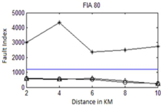
Fig7. Variation of fault index from Bus2 at LG Fault on Phase AG for transmission line at Fault Inception Angle  $80^{\circ}$ .
