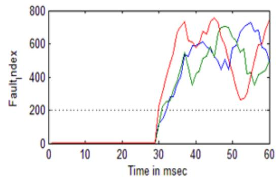
Fig13 Detection of LLLG fault at PV generation.
