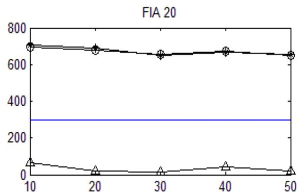
Fig 5. Variation of fault index from Bus1 at LL Fault on Phase AB for transmission line at Fault Inception Angle 20°.
