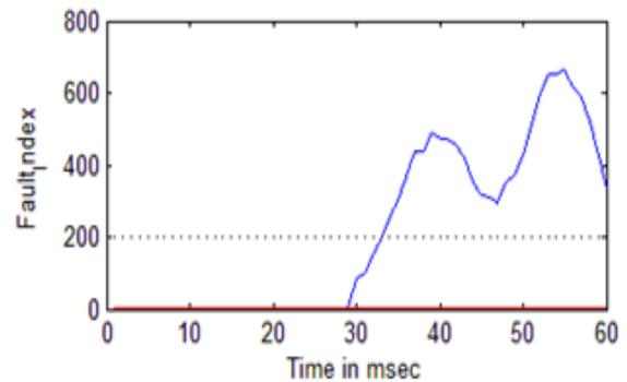
Fig 12 Detection of LG fault at PV generation
