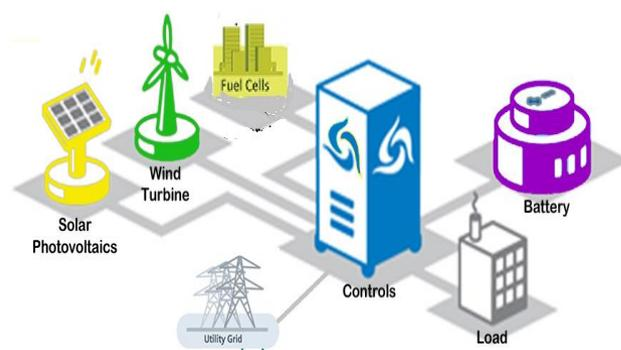
Fig 2: Microgrid connected energy resources to utility grid
