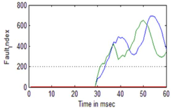
Fig 11: Detection of LLG at wind generation
