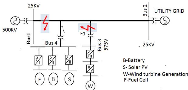
Fig 3. Single line diagram for microgrid connected to utility grid
