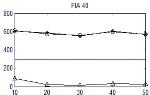
Fig 6. Variation of fault index from Bus1 at LL Fault on Phase AB for transmission line at Fault Inception Angle 40°.
