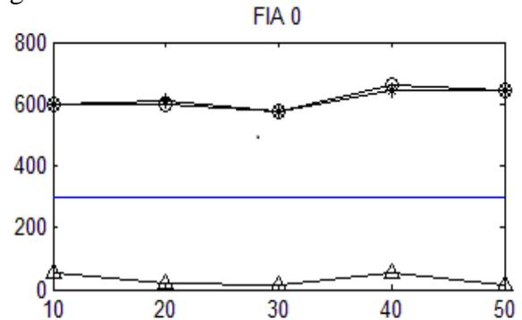
Fig 4. Variation of fault index from Bus1 at LL Fault on Phase AB for transmission line at Fault Inception Angle 0°
