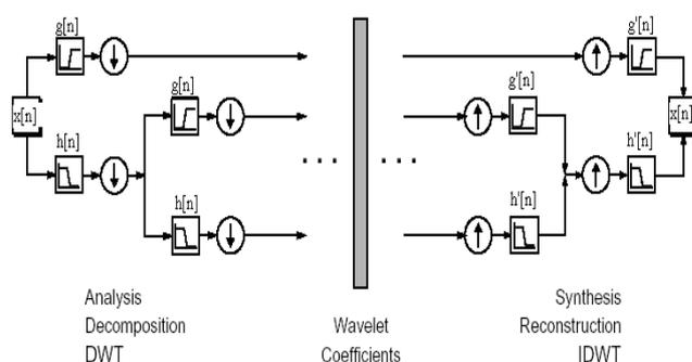
Fig 1. Analysis of signal using wavelet transforms
