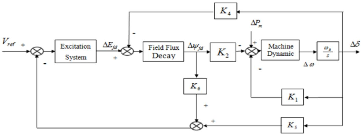
Fig.2 Block diagram of one machine infinite bus system
