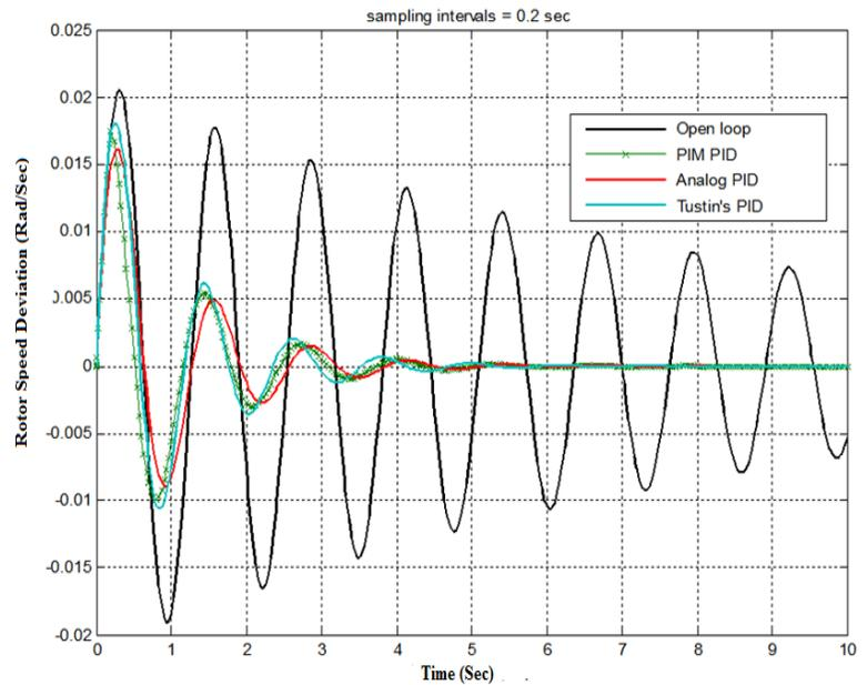
Fig. 7 Dynamic responses to step change in the mechanical torque (sampling interval 0.2 s) of PID controller.
