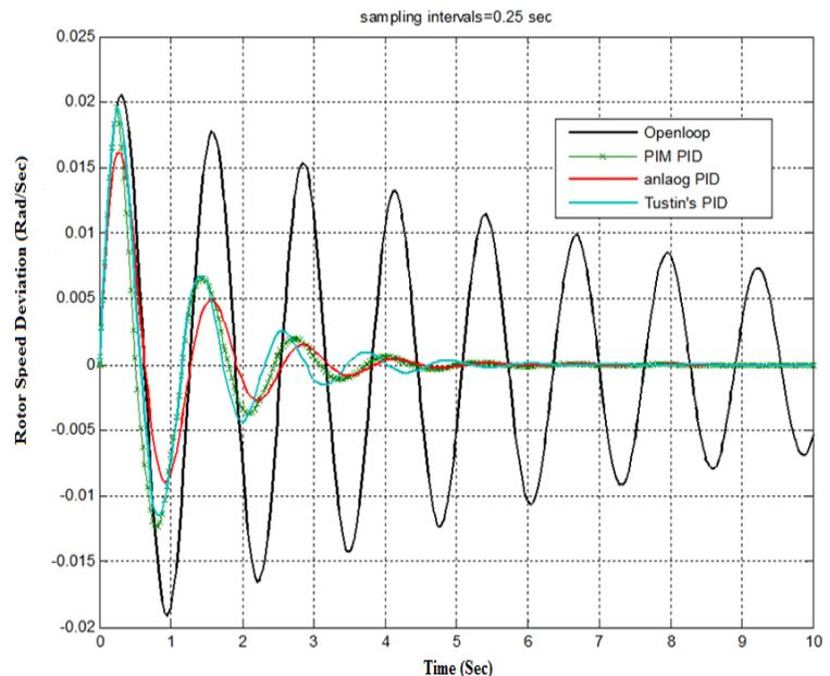
Fig. 8 Dynamic responses to step change in the mechanical torque (sampling interval 0.25 s) of PID controller.
