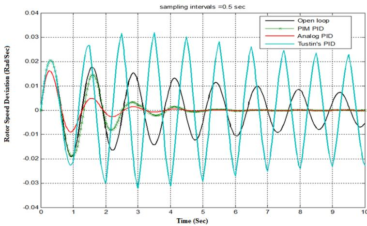
Fig. 10 Dynamic responses to step change in the mechanical torque (sampling interval 0.5 s) of PID controller.
