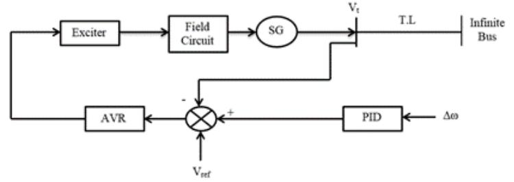
Fig. 1 Schematic of a single-machine infinite-bus (SMIB) power system.
