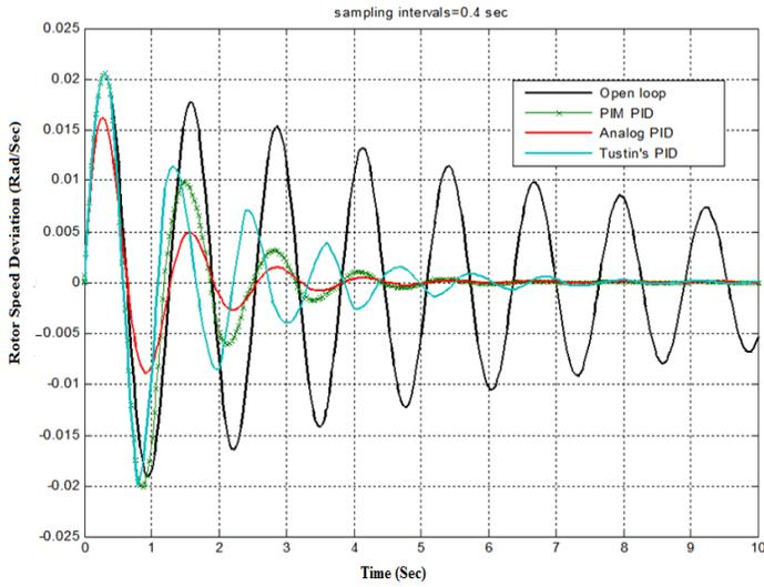
Fig. 9 Dynamic responses to step change in the mechanical torque (sampling interval 0.4 s) of PID controller.
