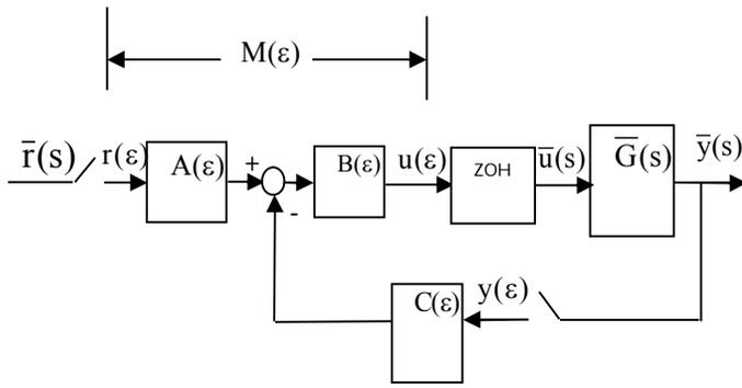
Fig. 5 Discrete-time control system redesigned using the PIM method.
