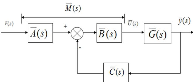
Fig. 3 Continuous-time control system.
